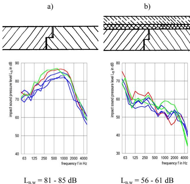
Figure 2: impact sound pressure level of timber floors
